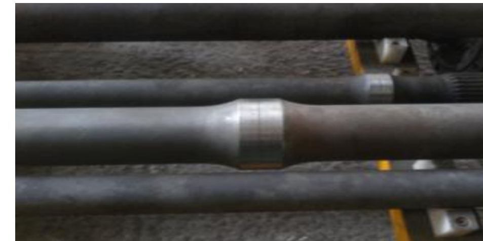
Groove caused by O ring
