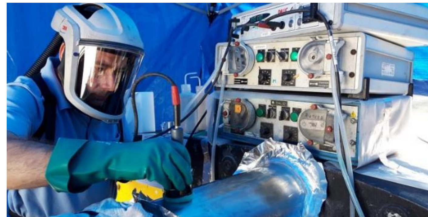
Groove repair on a rudder shaft
