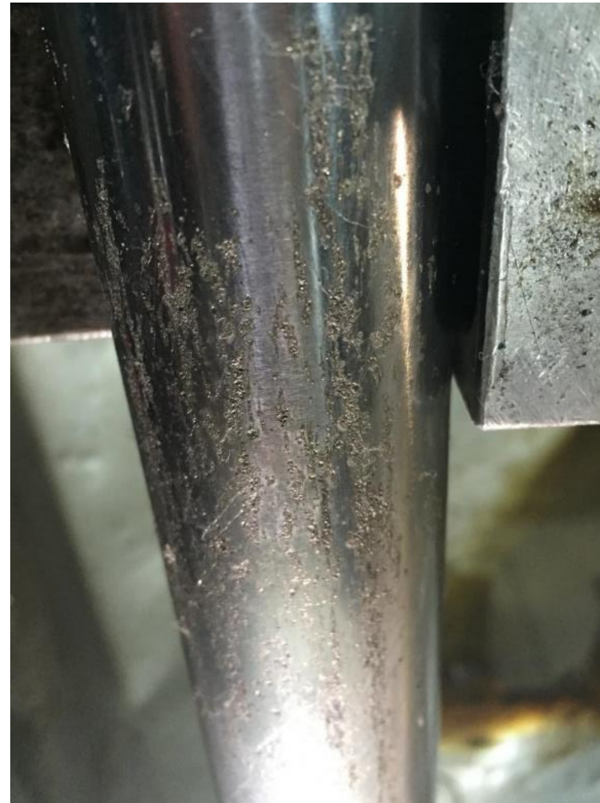
All the surface of the jack needs to be rebuilt → Tank plating
