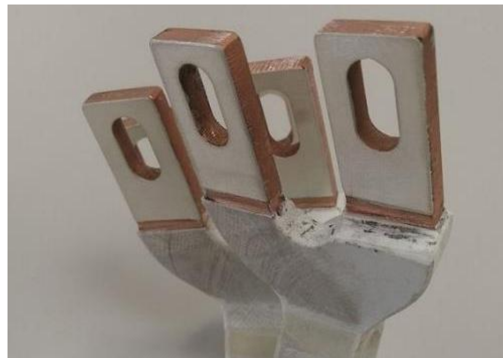
Silver plating on bus bars for electric conductivity
