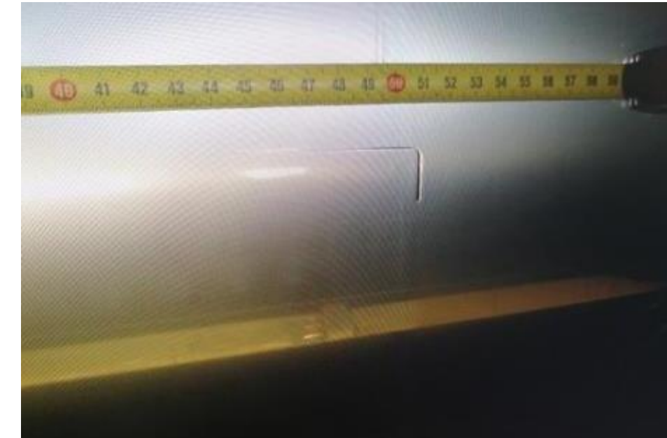
Impact Allen Key on printing cylinder
