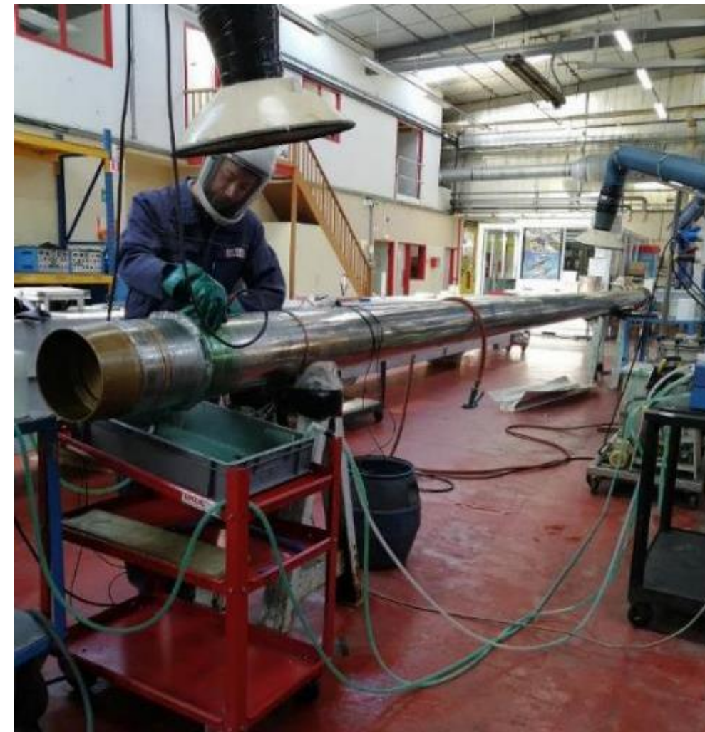
Corrosion protection on a submarine mast
