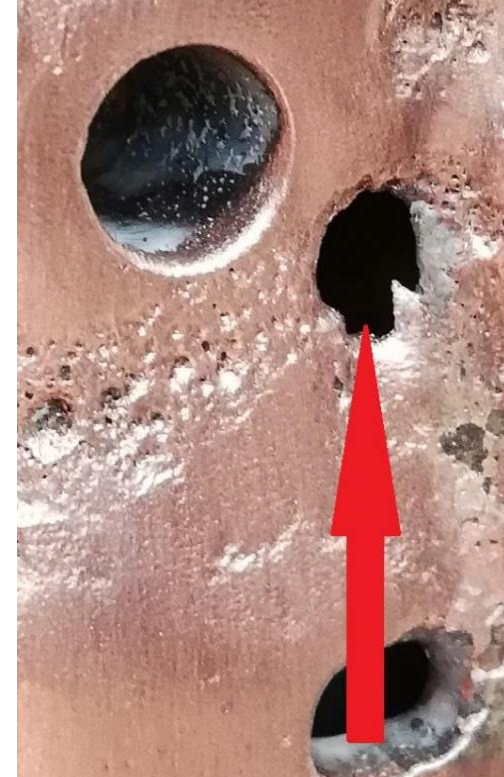
Many porosities on several millimeters thickness
